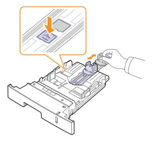
After inserting paper into the tray, adjust the support guide so that it lightly touches the paper stack.
